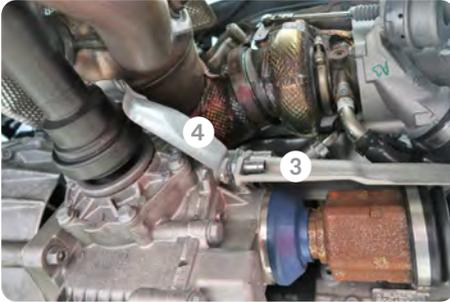
3. Separate the flange connections between the downpipe and the exhaust system.
